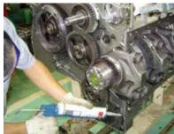
Diesel Engine Side Cover Sealing
