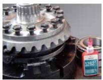
Differential Mechanism Thread Locking
